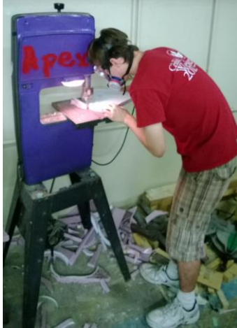
Figure 41– Cutting with bandsaw
